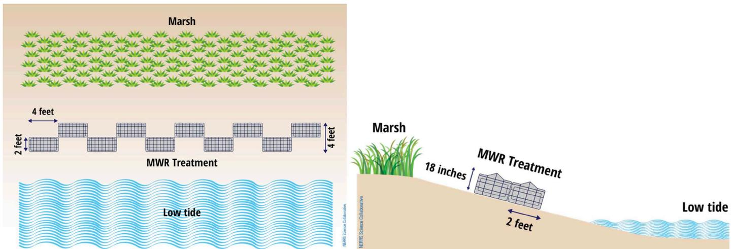
**Figure 3.8.** Overhead (left) and cross section (right) views of a typical manufactured wire reef (MWR) design in the intertidal zone used for this study.
