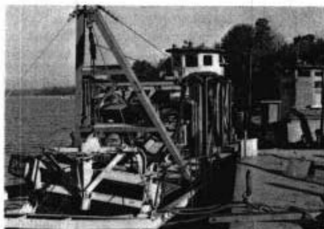
FIGURE 18—Mechanical intertidal oyster harvester now under development by the Ladies Island oyster canning plant.
