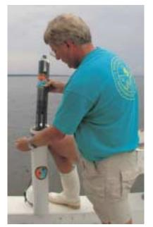
Continuous data collectors are deployed for 25 hours at each station to better evaluate water quality conditions over multiple tidal cycles.
