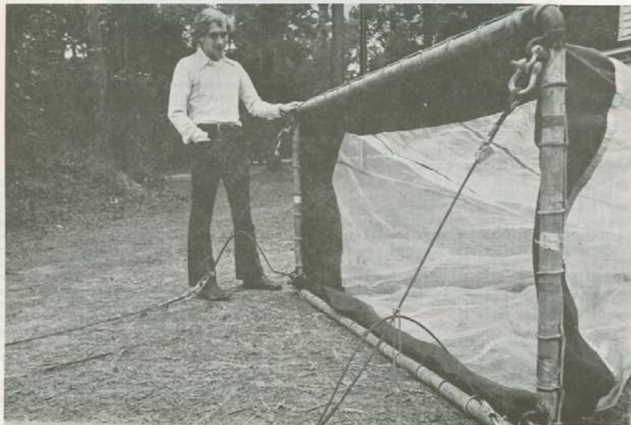
Figure 1. Standard Boothbay neuston net 1 x 2 m with pipe frame.
